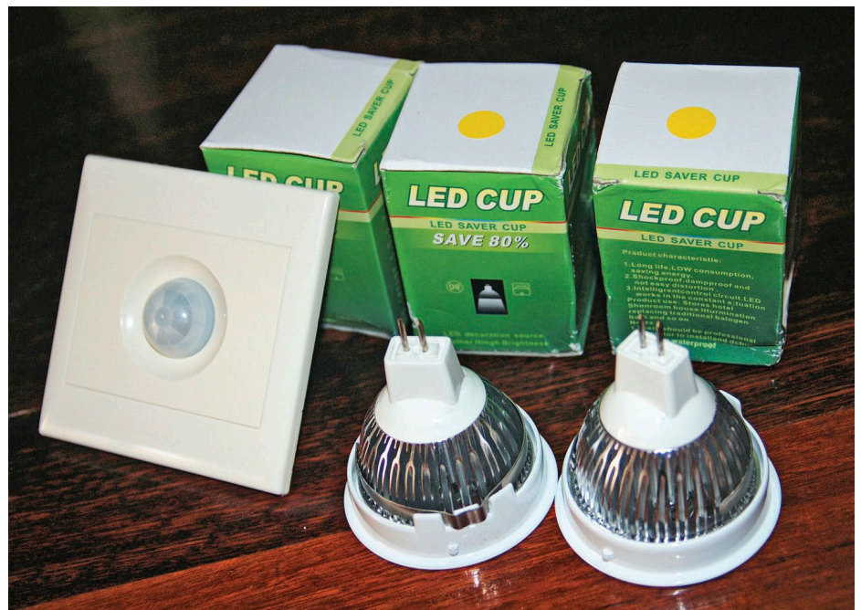
↑ Low cost MR16 LED bulbs are readily available on eBay, as is a range of 12 volt control gear like the passive infrared sensor at the left of the photo.
