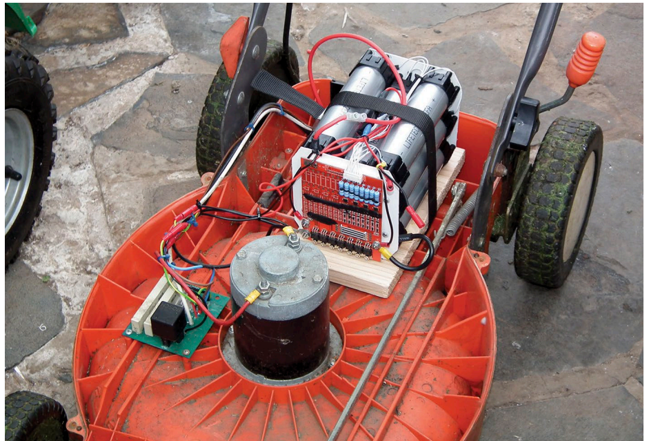
↑ The mower, minus cover, with the new battery fitted. The two bullet sockets on the right go to a volt meter mounted in the cover.
